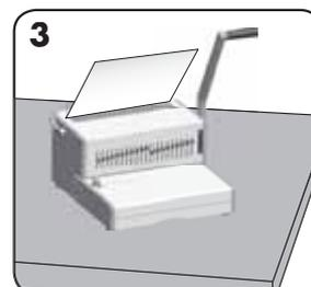
Load punched sheets directly onto the opened comb. Starting with the front of the document.
