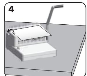
When all punched sheets are loaded onto the comb, push the comb lever backwards to close the comb and remove the bound document.
