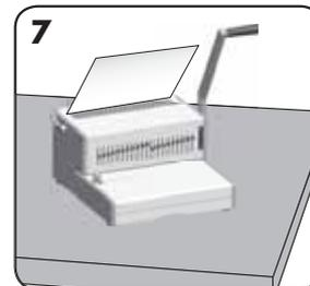
Load punched sheets directly onto the open comb.
